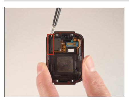
Use a pair of tweezers to remove the rubber gasket. It should come off with ease.
