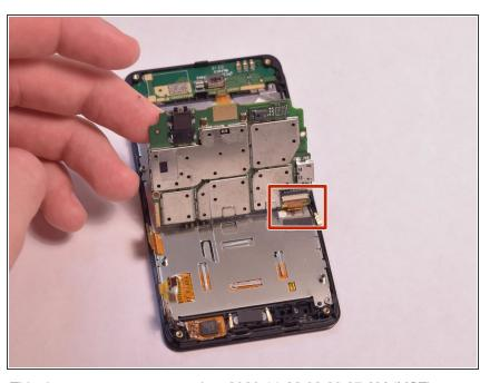
Lift the motherboard and remove the connector on the back by using the tip of a spudger or your fingernail to flip up the small retaining flap. Then pull the ribbon cable out.
