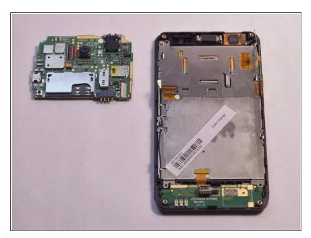
Remove the motherboard from the device.
