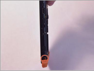
Remove the two 5mm T4 screws on the sides of the small orange plate.
