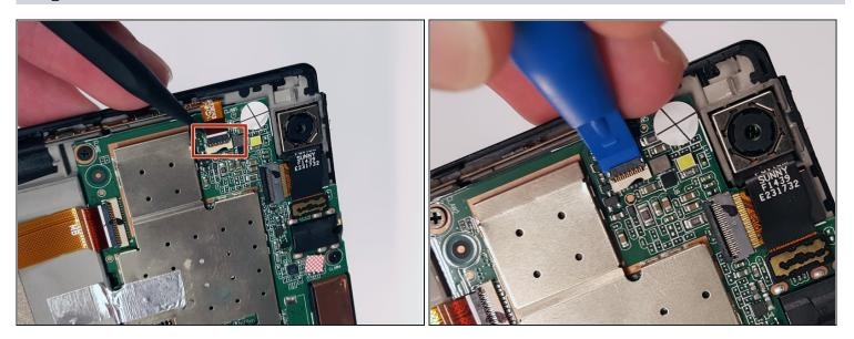
• Use the tip of a spudger or your fingernail to flip up the small locking flap. Then, you can safely pull the cable out from under the camera.
