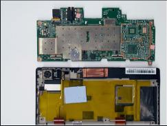
Use the spudger to gently pry the motherboard out of the frame from each side.
