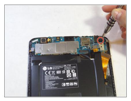
Remove all the 3mm silver screws and the 2mm black screws on the motherboard and carefully lift it out of the device.
