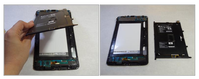
• Unhook the battery from the top of the device.
