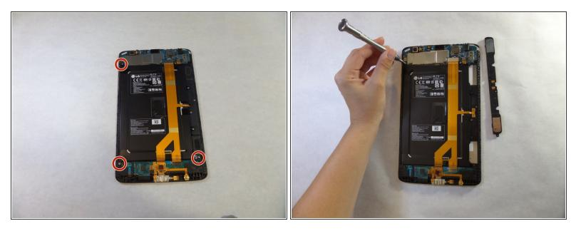
• Remove the 3mm Phillips #000 screws from the corners of the battery.
