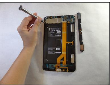
Remove the 3mm Phillips #000 screws from the corners of the battery.
