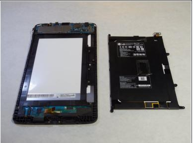
Unhook the battery from the top of the device.
