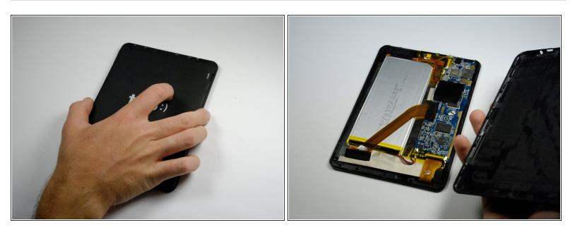
• Remove the back panel from the rest of the tablet and set it aside.
