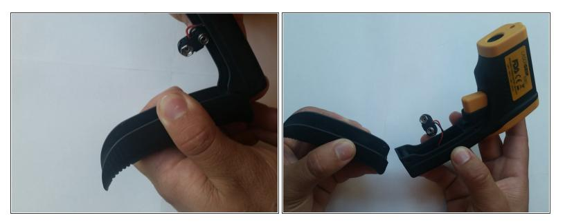
Remove the battery cover from the device by pulling it straight out.
