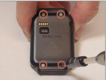
• Use a T5 Torx Screwdriver to remove the 4 (0.4 mm) screws located on the back of the watch.
