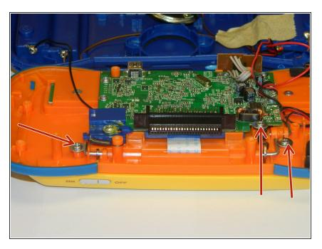
Remove the three 4.0 mm Philips J0 screws holding the "L" shaped brackets in place.
