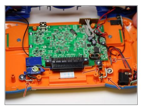
Remove the three "L" shaped brackets and the spring.
