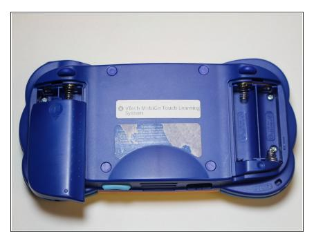
Remove the battery covers and the four batteries.
