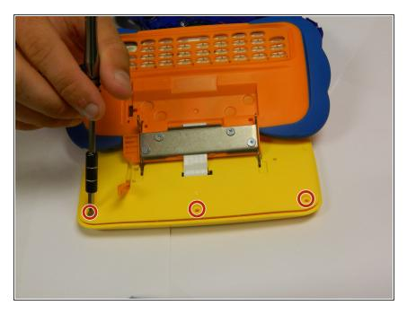
Flip the device over and remove the three 4.0 mm Philips J0 case screws.
