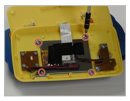
Remove the 4 (3.4 mm Philips J0) screws holding the screen in
