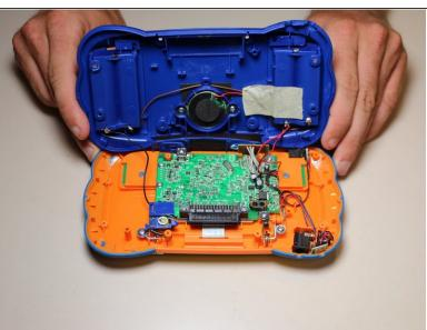
Using a plastic opening tool, separate the two pieces of the case carefully.
