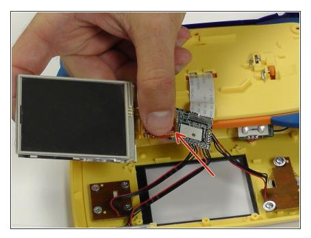
Peel the ribbon wire off of the circuit board. Now the screen should be free to remove.
