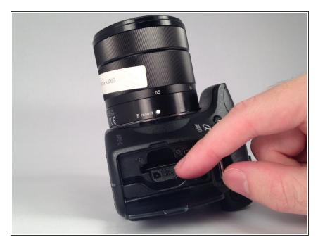
Depress the old memory card to release it from its cradle. Extract the card and replace it with the new one, pushing the card in until it locks.
