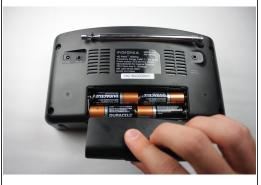
Remove the panel on the back side of the radio by pressing the arrow in a downward motion.
