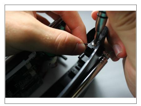
Using the J1 Philip's head screwdriver, unscrew the bolt attaching the antenna to the back panel.
