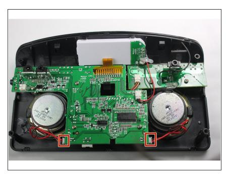
Using the needle nose pliers or regular pliers, separate the wire connectors attaching the speakers to the circuit board on its right and left side.
