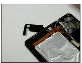
• Use your fingers to remove the plastic L-shaped speaker housing from the tablet.
