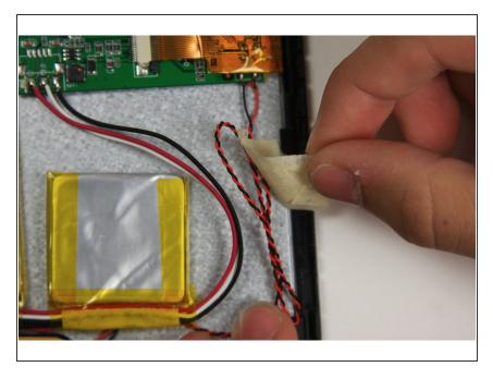
Remove the masking tape covering black and red wires that connect the speaker to the right side of the bottom of the motherboard.
