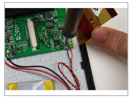
Desolder the red and black wires on the right side of the motherboard that connect the speaker to the motherboard.
