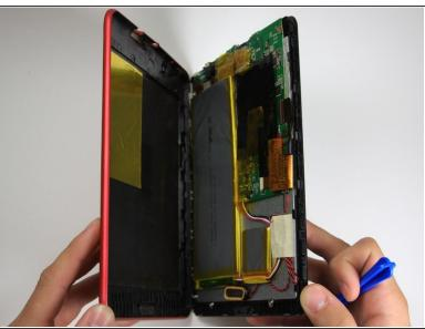
Use your hands to completely separate the rest of the front glass from the back panel.
