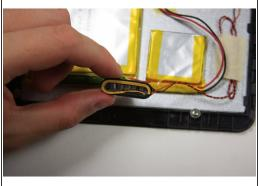
Using the flat end of the spudger, remove the speaker from the device by sliding the spudger underneath the speaker.
