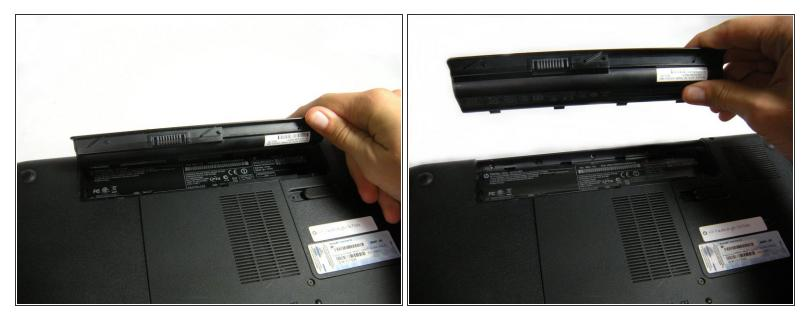
• Lift the battery from its compartment away from the laptop.
