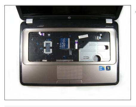
With the ribbon cable detached, you can now completely remove the keyboard.
