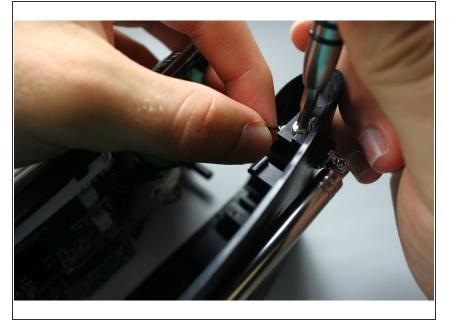
Using the J1 Philip's head screwdriver, unscrew the bolt attaching the antenna to the back panel.
