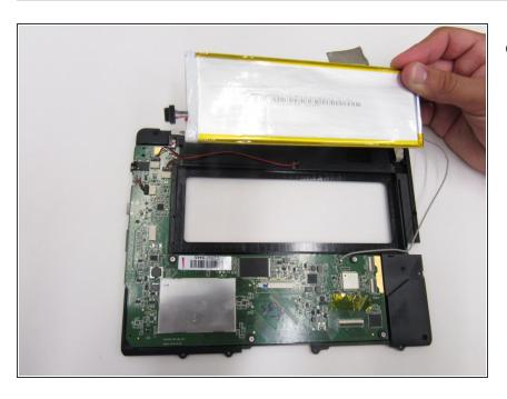
Remove the battery from the circuit board by lifting it with the spudger or finger.
