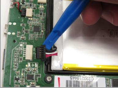
Wedge a plastic opening tool in between the male, black module and female, white module to disconnect the wires module from the circuit board.
