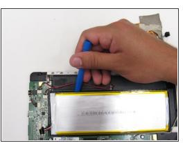
Use a plastic opening tool to pry the battery from the circuit board by wedging it around the perimeter of the battery.
