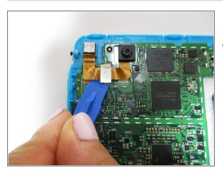
Remove the flat-topped connector that connects the cameras to the motherboard by using the plastic opening tool to pry up on each side.
