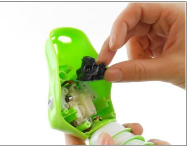
Carefully push the sensors out of the nose socket with your fingers.
