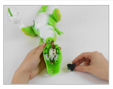
Remove and replace the nose sensor. To reassemble your device, follow these instructions in reverse order.
