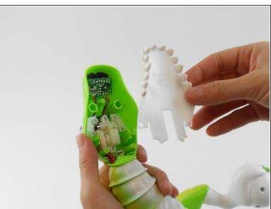
Remove the roof of Zoomer Dino Boomer's mouth by unscrewing the 7.5 mm Phillips #0 screw.
