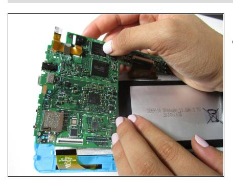
Remove the motherboard by lifting it out of the casing. To reassemble your device, follow these instructions in reverse order.
