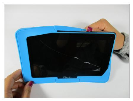
Remove the rubber case by beginning to peel from one of the top corners and continue peeling until the cover is completely removed.
