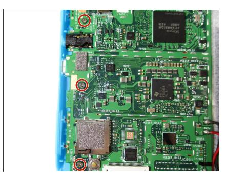
Unscrew the three 4 mm screws with a Phillips #000 screwdriver.
