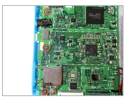
Remove the three 4 mm screws on the motherboard with a Phillips #000 screwdriver.
