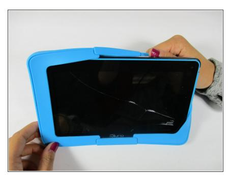
Remove the rubber case by beginning to peel from one of the top corners and continue peeling until the cover is completely removed.
