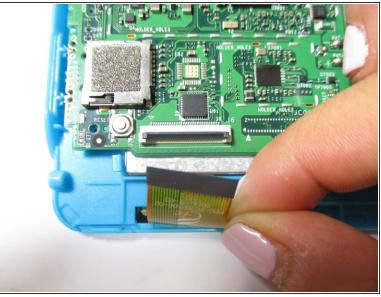
Remove the orange data display ribbon wire to the left of the battery by prying open the ZIF connector with the plastic opening tool.
