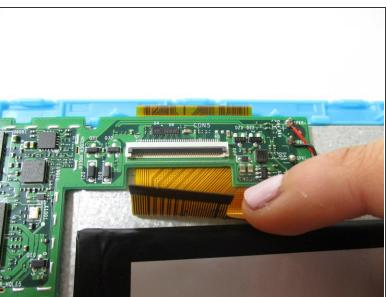
Remove the orange data display ribbon wire above the battery by prying open the ZIF connector with the plastic opening tool.
