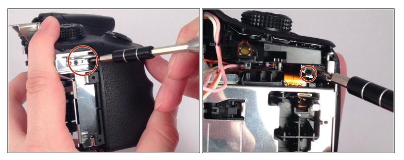
• Remove the three remaining screws holding in the protective metal casing.
