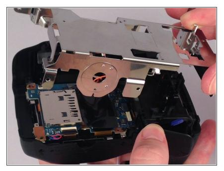
• Remove the metal casing.
