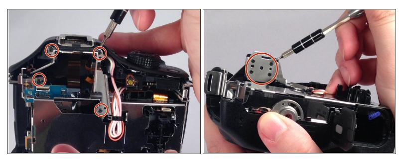
• Remove the eight screws securing the mount for the flash device.
