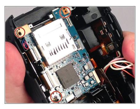
• Remove three screws holding down the motherboard .
