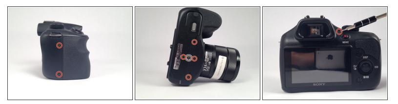
• Remove the seven highlighted screws shown here.
