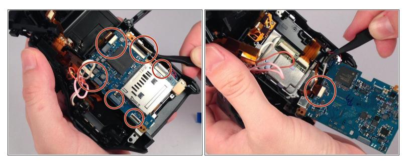
Detach the nine serial cables connecting it to the camera body.
