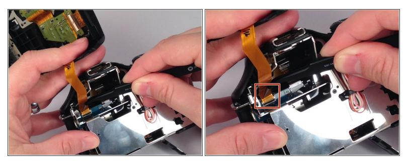
• Gently but forcefully lift up on the parallel cable connecting the two halves of the camera.
