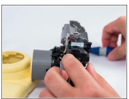
Locate the photo-flash capacitor, then find all the connecting wires to the motherboard and battery compartment. Take notes to which exact wires they are to limit mistakes.
