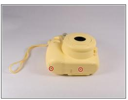
Remove screws from bottom of camera with a small #00 Phillips Screwdriver. Then remove screws around the camera. Additionally, there are two screws in the battery compartment which also need to be removed.
