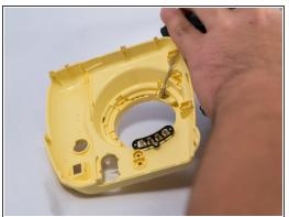
Once all screws are removed, gently pry open the front casing with your hands or plastic opening tools carefully. Do note that there will be a spring that attaches the front casing and the main circuit board, so refrain from allowing excess tension on the spring.
