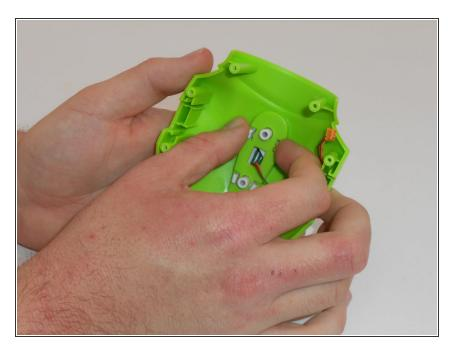
Where the button is largest, squeeze the two white tabs together.
