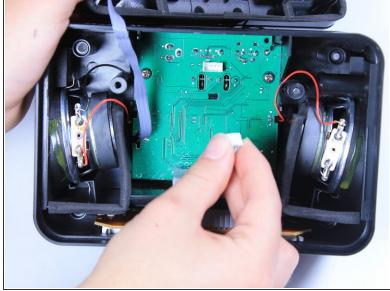
Grip the white ribbon cable connector that attaches the lightning cable to the middle of the central circuit board located in the bottom of the clock. Pinch and pull straight up to detach the cable.
