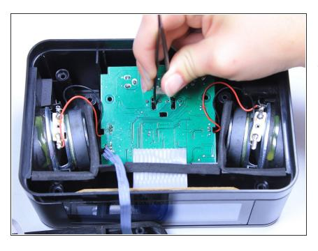
Once the ports on the back of the circuit board are displaced and resting against the back of the clock, use a pair of tweezers to lift the circuit board up off of the bottom of the clock, continuing to feed the radio antenna through the side of the clock as the board lifts up.
