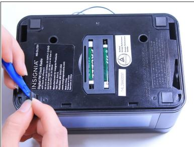
Lift the four adhesive covers on each of the corners on the bottom of the clock using a plastic opening tool or your fingernail.
