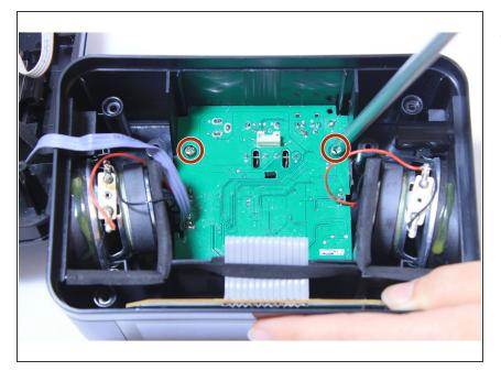
Unscrew the two 10mm screws from the bottom circuit board.
