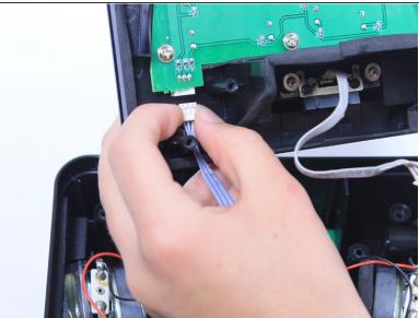
Remove the white ribbon connector that connects the central circuit board to the circuit board attached to the top of the clock by gripping it on both sides and pulling it straight away from the board.
