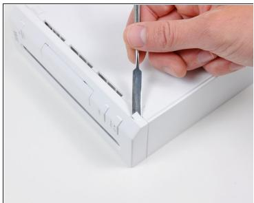
• Use a metal spudger to remove the white plastic screw covers stuck to the lower case near the front of the Wii.
