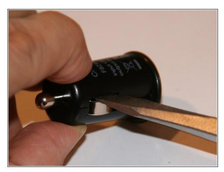
Pry space between ground contact and plastic casing, using a large flat blade screwdriver. Alternate prying on both ground contacts on either side of the case. The case should begin separating at the USB side of the adapter.
