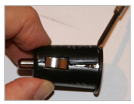
Use a smaller flat blade screwdriver to pry on the gap created between the side and the USB "front" of the adapter. Eventually you can use your hands to pull the two casing halves apart.
