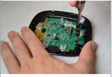
• Use the PH00 screwdriver bit to unscrew the three 4mm Phillips screws on the control board.
