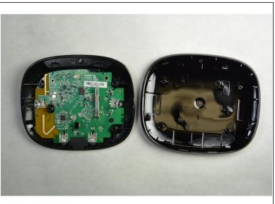
Use a spudger to separate the top and bottom pieces of the device.
