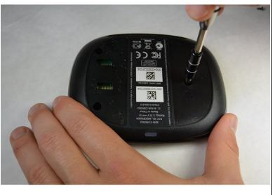
• Use a PH00 screwdriver bit to remove the four 6mm Phillips screws on the bottom of the device.
