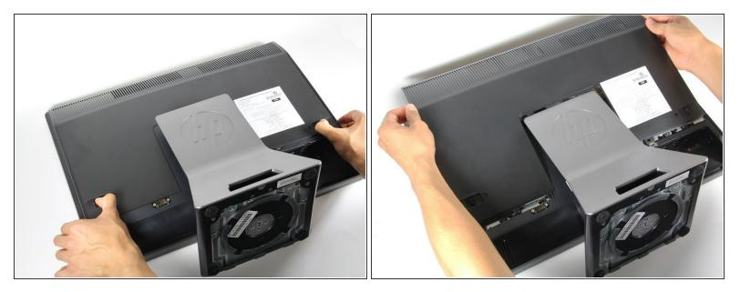
• Push the unlock tabs on the back on the monitor in and towards each other while sliding the back cover up.
