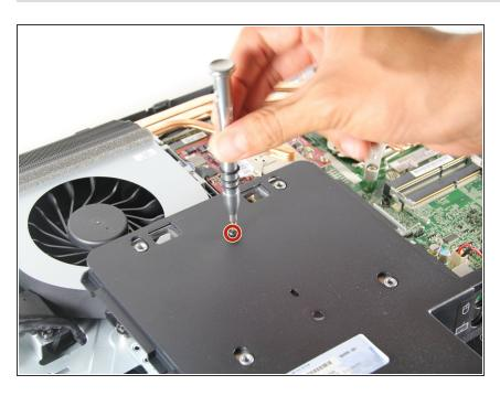
Take out the single 3/8" screw, with the T15 Torx Screwdriver, from the middle of the backplate.
