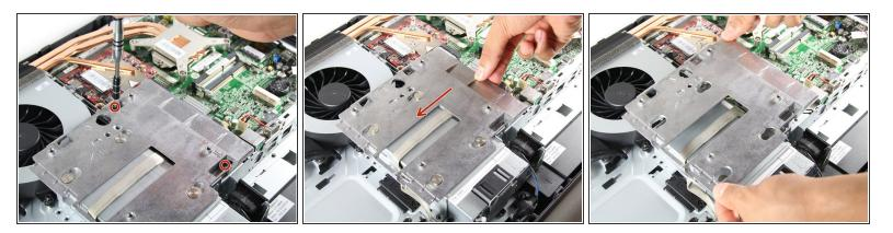
Remove both 3/8" screws using the T15 Torx Screwdriver from the metal plate, and slide the plate to the left.
