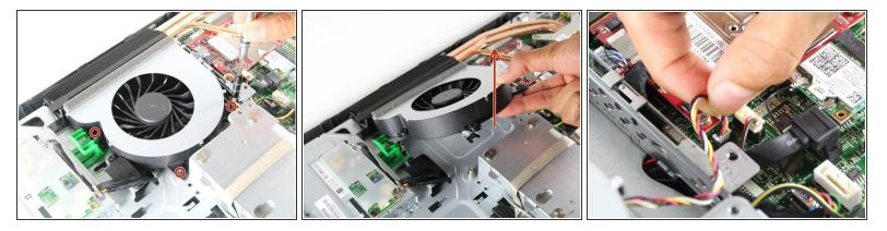
Unscrew three surrounding 1/4" screws, with the T15 Torx Screwdriver. Pull out the fan and attached wires.
