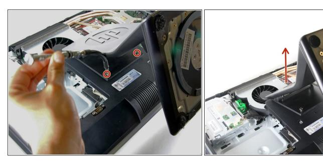
Loosen the two 1/2" screws, with the T15 Torx Screwdriver, on each side of the stand. Remove stand.
