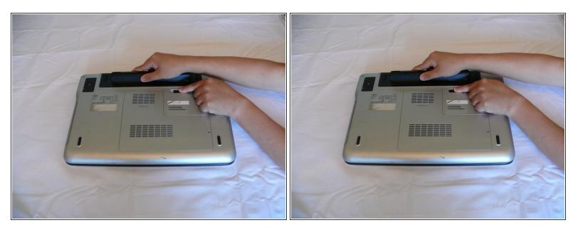
• Slide the tab below the battery to the left and hold the tab in place.
