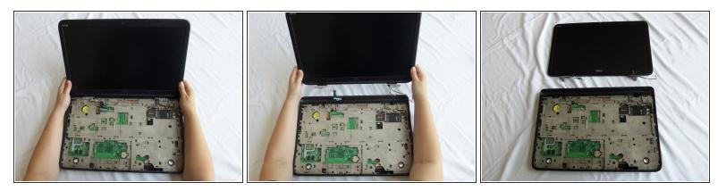
• Hold the plastic edge of the display firmly and lift to remove the display.
