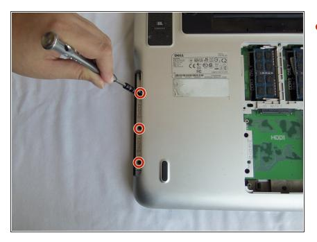
Unscrew three 4mm screws near the edge of the optical drive compartment with a Phillips screwdriver.
