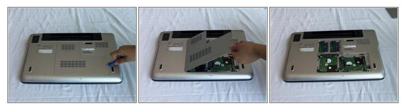
Lift the module cover by inserting a plastic opening tool into the crevice near the screw and lift upwards.
