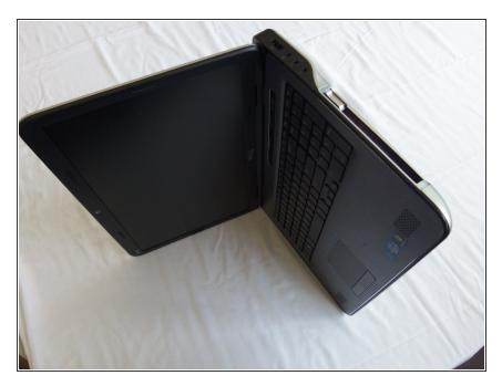
Open the laptop to about a 90 degree angle and place it on its side with the empty optical drive slot pointing upwards.
