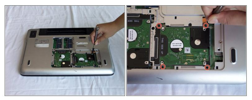
• Remove the four 4mm Phillips screws fastening the first hard drive.
