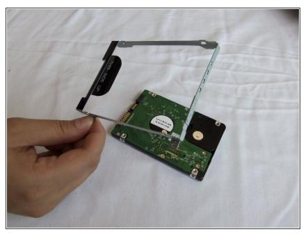
• Remove the hard drive casing.
