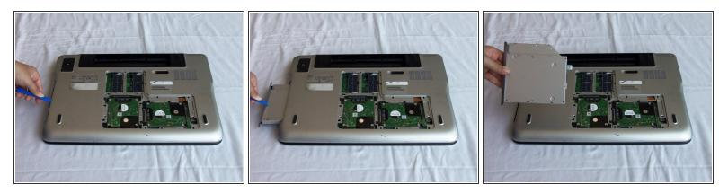
• Using a plastic opening tool, pull out the optical drive.
