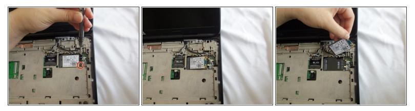
• Unscrew the 4mm screw from the WWAN card with a Phillips screwdriver. The card will lift itself.
