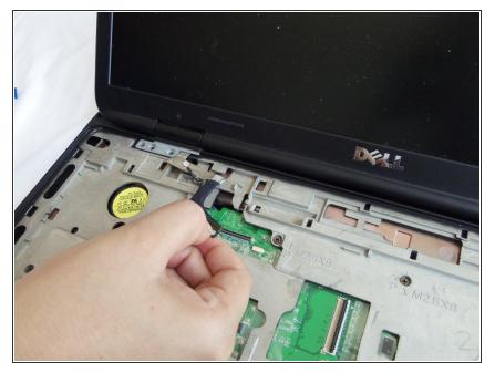
• Gently remove the monitor cable from its holdings from the board.
