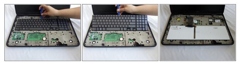
• Using the plastic opening tool, slightly lift and rotate the keyboard until it's upside down from the display side of the laptop.
