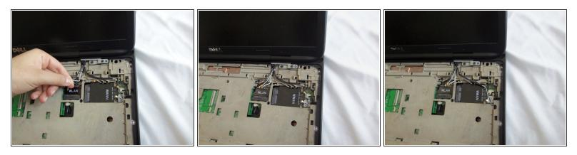
• Gently remove the wires for the WLAN and WWAN cards from their housing.
