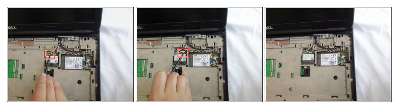
Insert the pointy side of the spudger below the golden connector of the white cable on the WLAN card and lift to detach.
