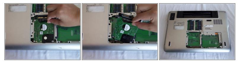
• Using the tab that says "THIS SIDE UP," pull away from the laptop to remove the hard drive.
