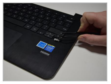
• Removed the loosened key with the tweezers.
