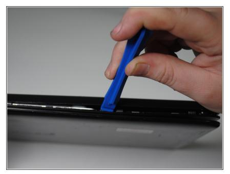
• Using a plastic opening tool, work around the Chromebook separating the plastic case at the seam.
