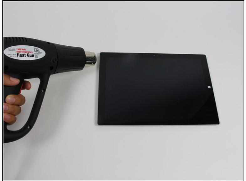
**!** Before you begin, discharge the Surface Pro's battery below 25%. A charged lithium-ion battery can catch fire and/or explode if accidentally damaged during the repair.
