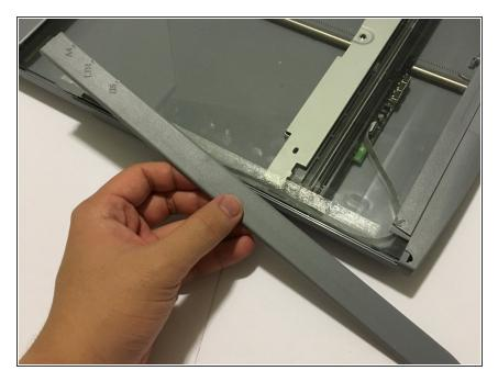
Once the adhesive strip is sliced through, the plastic bar that is attached should release. Set aside the plastic bar.
