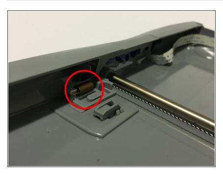
Locate the small metal spring behind the front buttons of the Canon CanoScan N670U.
