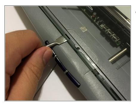
Insert the metal spudger tool underneath the glass scanner bed.
