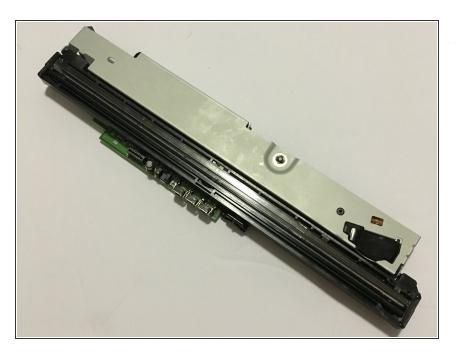
Remove the sensor bar from the scanner and replace it with the new one.
