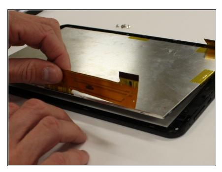
Once the screen is pried free from the digitizer, simply grab the thin orange circuit strip and carefully pull in an upwards motion to remove the screen from the digitizer. Set screen to the side.
