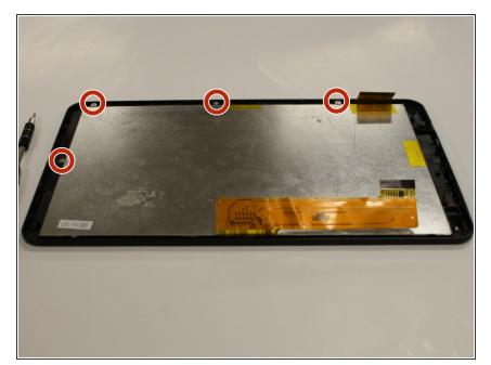
Begin by locating the four 3mm silver screws that are holding the screen down to the digitizer. Set screws to the side.
