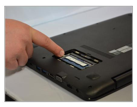
With your finger, push the two metal tabs (one on each side) outward until the RAM card pops up.
