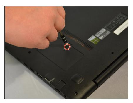
Using a #0 Phillips screwdriver, unscrew the single 2.5mm screw on the RAM cover.
