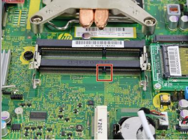
When replacing the RAM stick, take note of where the small notch on the stick is and where there is a similar notch on the slot. Make sure you position the new stick so that the notches line up.
