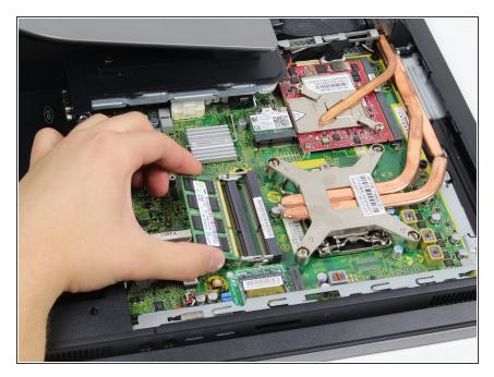
Gently pull the RAM stick up at an angle. You may need to wiggle the stick up and down or side to side in order to get it loose.
