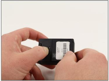
Push the tab on the back of the device left to remove the plate covering the battery.
