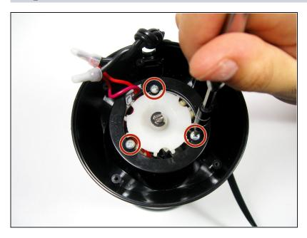
Remove the three 11.0 mm Phillips head screws surrounding the white fan blade on the base using the Phillips #1 screwdriver.
