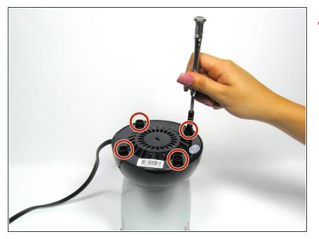
Remove the four 14.0 mm Phillips head screws in the feet of the base of the Magic Bullet using the Phillips #1 screwdriver.
