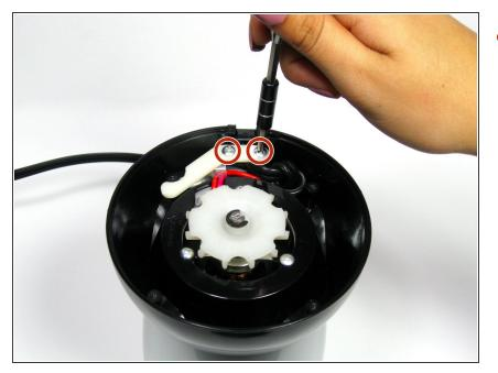
Remove the two 13.0 mm Phillips head screws from the white plastic cable guide using a Phillips #1 screwdriver.
