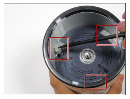
• Remove the three white rubber spacers with the spudger.
