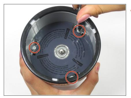
Remove the three 11.0 mm Phillips head screws using the Phillips #1 screwdriver.
