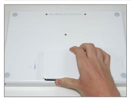
Lift the battery out of the computer.
