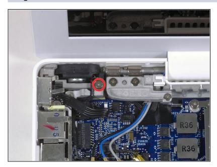
Remove the single Phillips screw securing the left speaker to the lower case.
