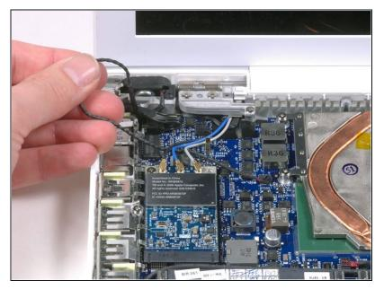
• Deroute the left speaker cable from beneath the Airport antenna cables.
