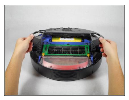
Lift up the back panel to remove it from the device.
