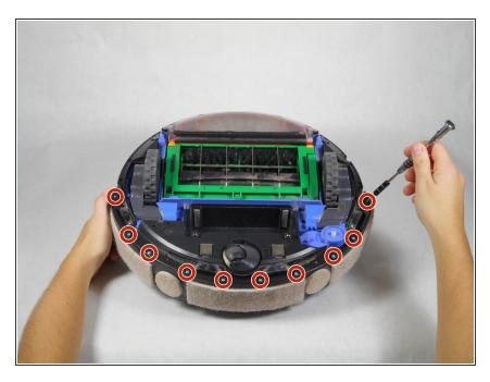
Using the Phillips #1 driver, remove the ten 10 mm screws on the bumper that run along the outer edge of the Roomba.
