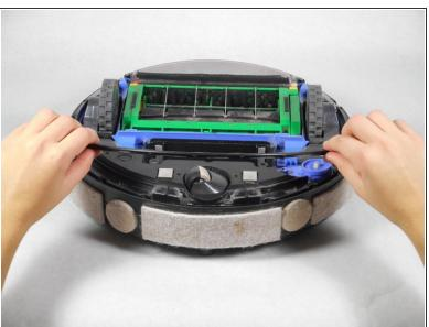
Lift the thin top cover that holds the bumper in place.
