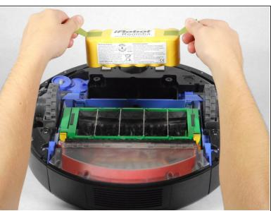
Lift up the yellow battery by pulling up the green tabs on its side.
