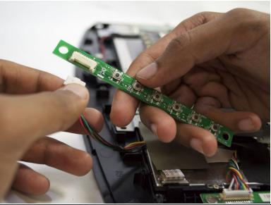
Detach the control button bar by depressing the small white tab that connects the bar to its wires.
