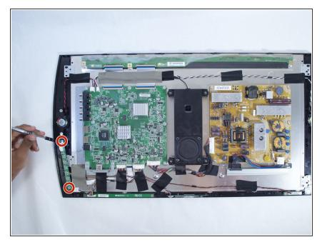
With the Phillips #01 screwdriver, remove the two 5 mm length x 7 mm head screws from the top and bottom of the control button bar.
