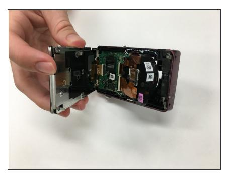
• Lift the metal plate away from the internal components of the camera
