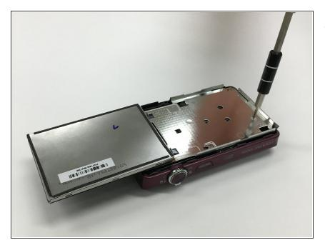
Remove the six designated screws sized 0.1 mm from the metal plate using a Phillip's Head screwdriver in size PH00.
