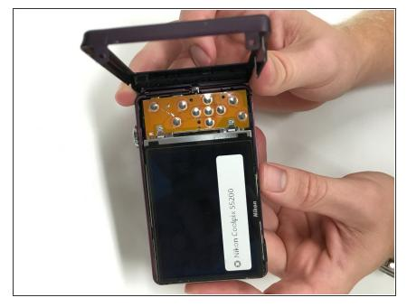
• Pull the plastic back cover off of and away from the LCD screen
