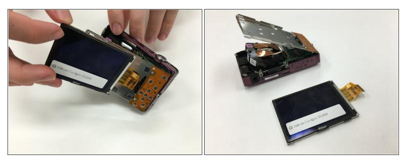
• Carefully remove the LCD screen by pulling it away from the camera. Repeat these steps in reverse order to install the new LCD screen.
