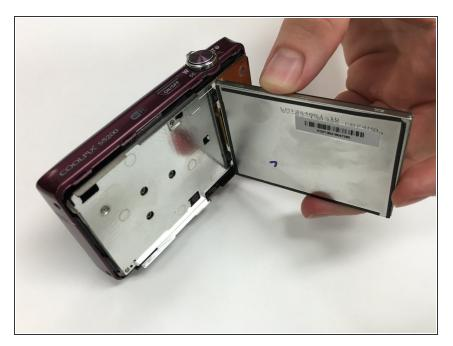
• Carefully remove the LCD screen from the silver plate that once held it in place by pulling it away from the internal components
