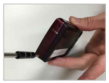
Use the Phillips Head screw driver head to remove the four 0.1 mm screws surrounding the outer edges of the camera
