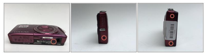
There are four 0.1 mm screws holding the front and back of the camera together all along the outside of the camera
