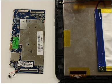
Carefully lift motherboard in a upward motion.
