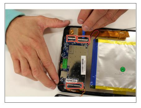
Using a plastic opening tool, gently pry up the three Zero Insertion
