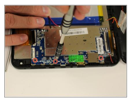
Using a J00 Philips screwdriver, unscrew the three black 4mm screws from the motherboard.
