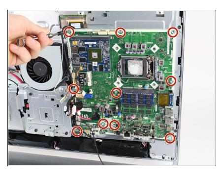
Remove the ten 7mm T15 screws from the motherboard.
