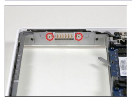
Remove the two Phillips screws attaching the battery connector to the lower case.
