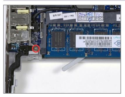
• Remove the single Phillips screw near the battery connector.
