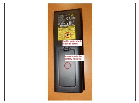
• There are two screws on this remote controller. One behind the yellow sticker. One in the battery housing.
