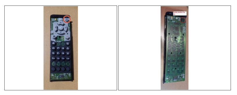
Using a spudger to ease the two pieces apart will help you get started. Pulling will most likely cause a break in the snap-in pieces.
