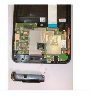
• Use the slender, metal spudger tool to gently lift up the edge of the speaker to remove the device.
